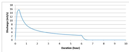
**Figure 11.** Direct Runoff Hydrograph of Siti Khodijah Retention basin
