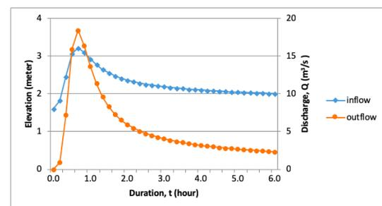
**Figure 13.** Inflow-Outflow Discharge of Hydrograph from HEC-HMS
