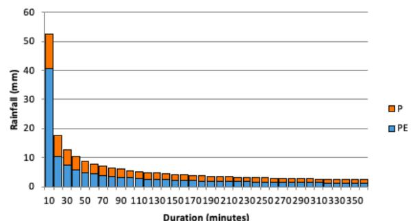
**Figure 9.** Correlation Graph between Rainfall and Effective Rainfall T-Return Period on Siti Khodijah Retention basin
