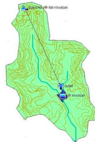
**Figure 12.** The Hydrology Model of Siti Khodijah Retention basin in HEC-HMS
