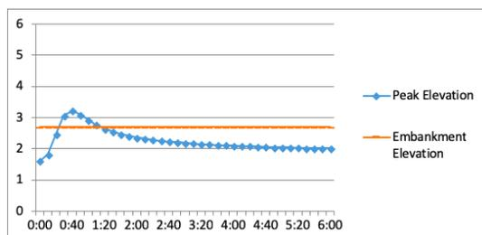
**Figure 14.** Comparative Graph between Simulated Peak Elevation and Embankment Maximum Elevation in Siti Khadijah Retention basin
