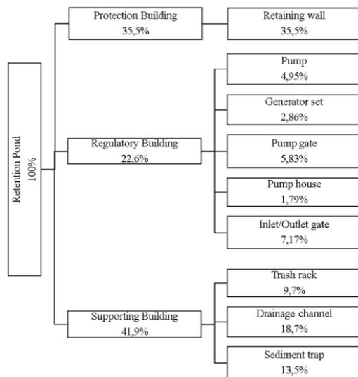
**Figure 2.** Value of each retention basin component
