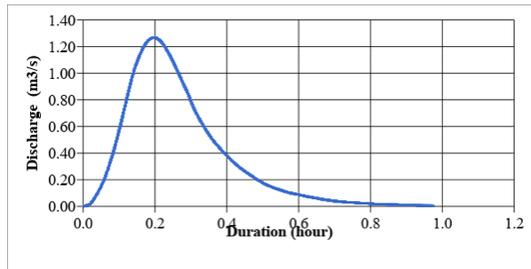
**Figure 10.** SCS Synthetic Unit Hydrograph of Siti Khodijah Retention basins
