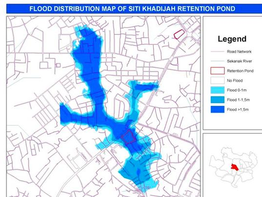
**Figure 15.** Flood Distribution Map of Classified Depth on Siti Khadijah Retention Basin
